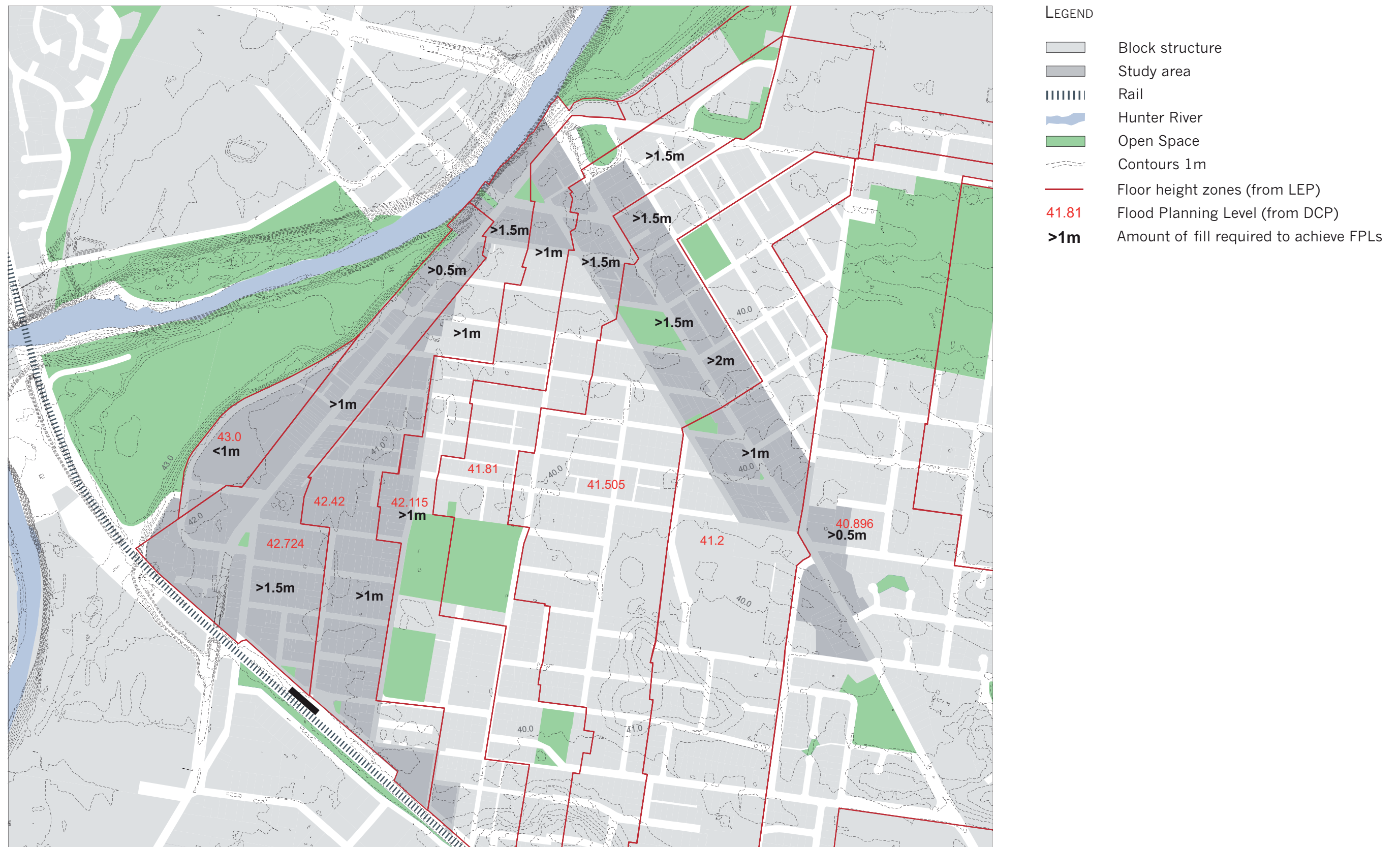
Illustration 2.10.1 Minimum finished floor levels (Flood Planning Levels) and elevation above natural ground, as per DCP 2012
